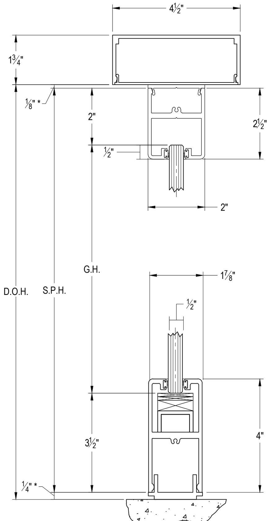
\* OPENING CLEARANCES MAY VARY BASED ON SITE CONDITIONS. STANDARD CLEARANCES SHOWN ARE USED IN FORMULA.
